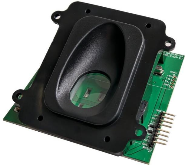
Fingerprint images and templates can be transferred between FS83C and host system for making flexible application. Futronic provides development tools to customer free of charge for integrating the FS83C with host system.
