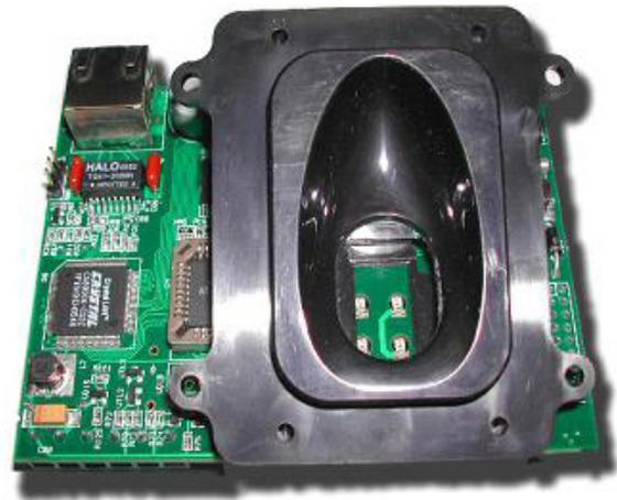
FS84C has 1 output channel (for external relay control) and 2 input channels (for door sensor and switch). So it can be used as a fingerprint access control device.
